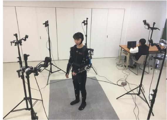
Fig. 3 Measurement by motion capture system
